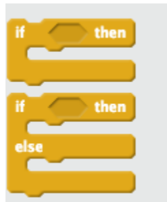
Figure 3.2: (Top) An IF block that only runs code if the condition slotted in the diamond shaped gap passes. (Bottom) An IF-ELSE block, in which the IF section works like the IF block and the ELSE section runs every time the IF section does not
